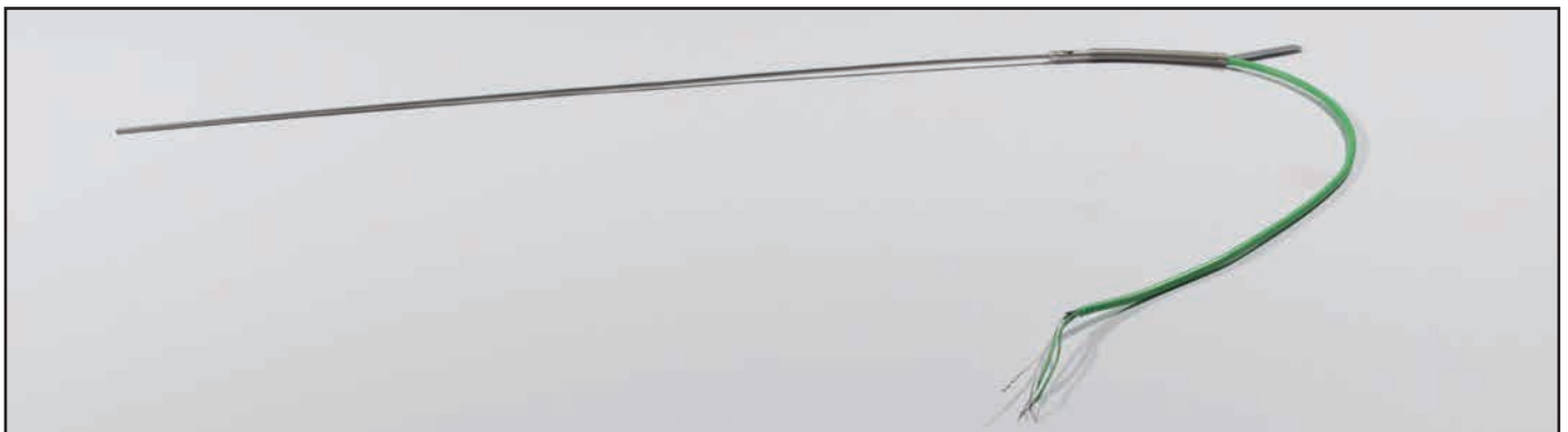
Mineral insulated thermocouple, Ø 3.0 mm, sheath material Inconel (2.4816), Model D
