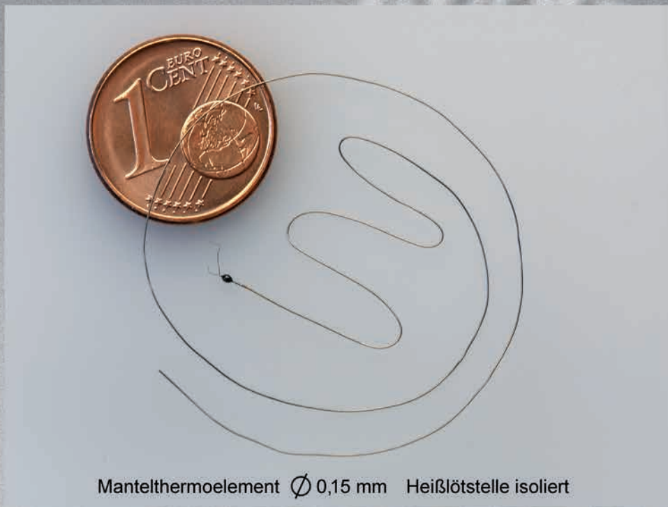
mineral insulated thermocouple Ø 0,15 mm with insulated hot junction
