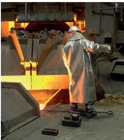
Temperature measurements in molten metals in a steel mill
